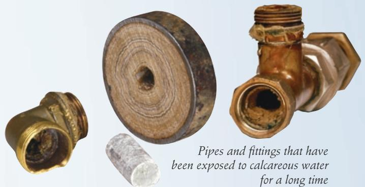
*Pipes and fittings that have been exposed to calcareous water for a long time*
